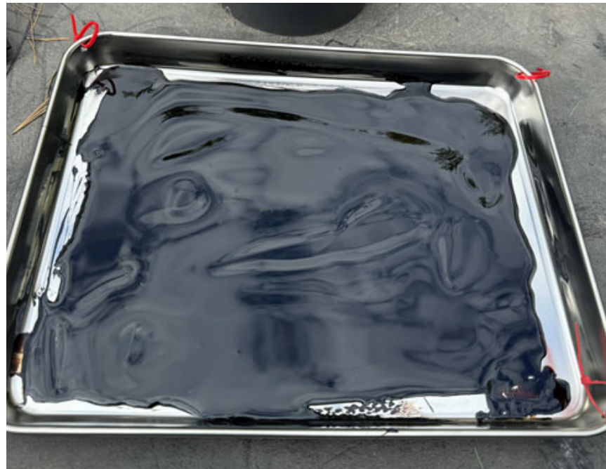
Figure 1. Stainless steel tray coated with weathered dilbit to create a target.
