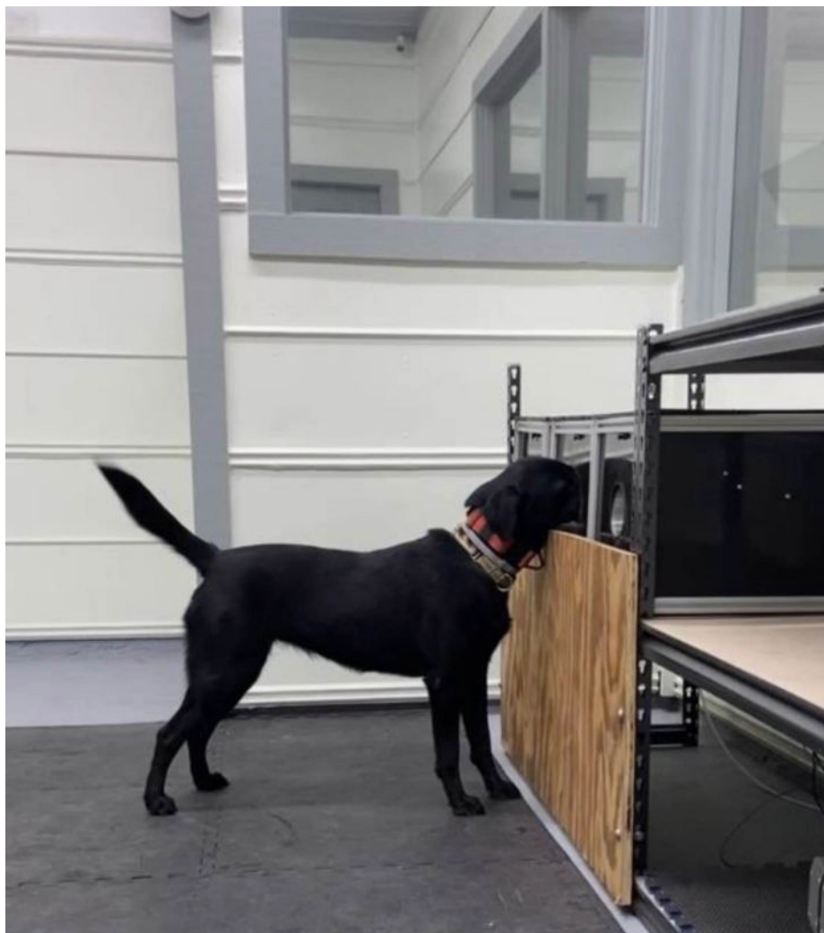
Figure 1. Dog alerting to an olfactometer port. Three olfactometers are aligned on a table. The dog is indicating the center olfactometer port is presenting a target odor and is engaging in a nose hold response.
