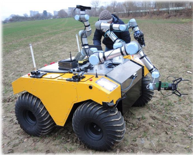
SNIFFBOT: search for leaks of dangerous gases
