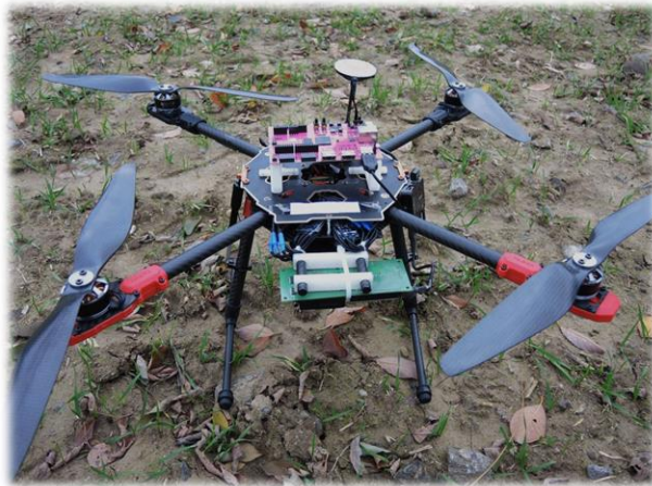
SNIFFBOT: search for leaks of dangerous gases
