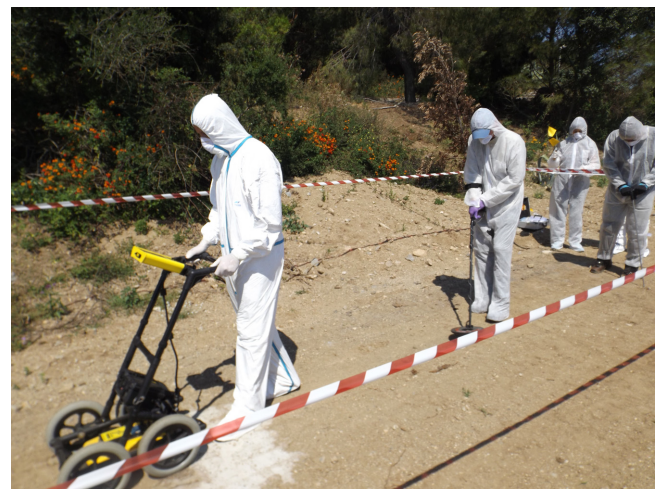
Figure 10. Geophysical search for a buried target. IUGS-IFG University of Messina, Sicily (Photo: Laurance Donnelly and University of Messina).
